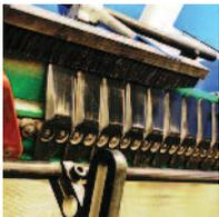
**Finishing:** Muller Martini six-station stitching line with cover feed.
